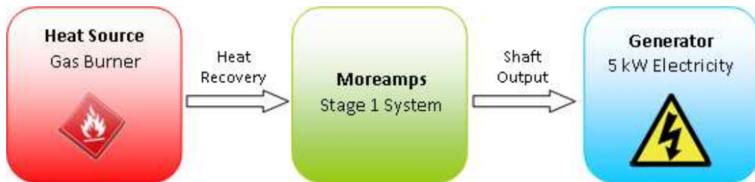
Figure 1 – Stage 1 (prototype system) overview.
